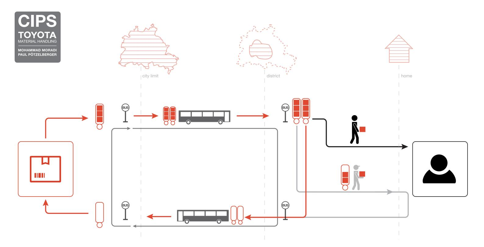
The parcelhub is located in the city outskirts and connected to the bus terminus. The parcels are packed into pods which attach to inbound busses like trailers.
